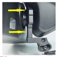
STEP 5 - Position the mount as far forward as you can. Tighten the clamp screw untill the Top and Mid Sections are slightly snug around the mirror stem.
