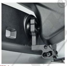
**STEP 6 -** Rotate the mount so it is parallel with the bottom of the mirror. Tighten the clamp screw untill the mount is securely attached to the mirror stem. Do not over tighten the clamp screw.
