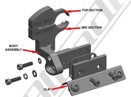
STEP 3 - Loosen the clamp screw so the top section seperates from the mid section. This will provide the necessary clearance to slide the mount over the mirror stem as shown above. Adjust the mirror paralell to the windshield and slightly upward for ease of installation.
