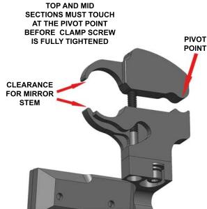
STEP 4 - BEFORE FULLY TIGHTENING THE CLAMP SCREW, MAKE SURE THE TOP AND MID SECTIONS ARE TOUCHING AT THE PIVOT POINT. If you can not get them to touch at the pivot point, you have an incompatible mirror type for this mount.
